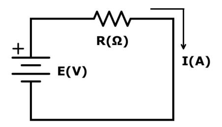
Figure 1. A simple electric circuit.
