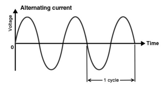
Figure 2. An alternating current (AC) waveform.
