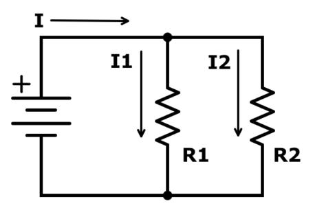
Figure 4. A parallel circuit.
