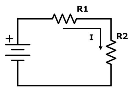
Figure 3. A series circuit.
