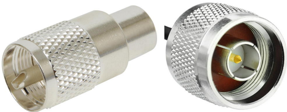
Figure 4-3. PL-259 connectors (left) are the most commonly used RF connector at HF and VHF frequencies, but N connectors (right) are better for use at frequencies above 400 MHz.
