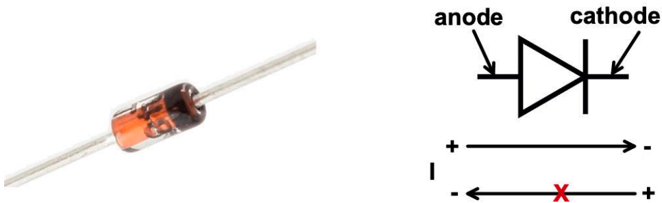
Figure 2-4. Diodes have two electrodes: the anode and the cathode. The cathode lead is often marked with a stripe on the package as shown above on the left.
