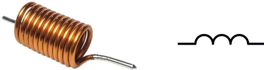
Figure 2-3. Inductors are typically coils of wire. The schematic symbol for an inductor (shown at right) looks like a coil of wire.
